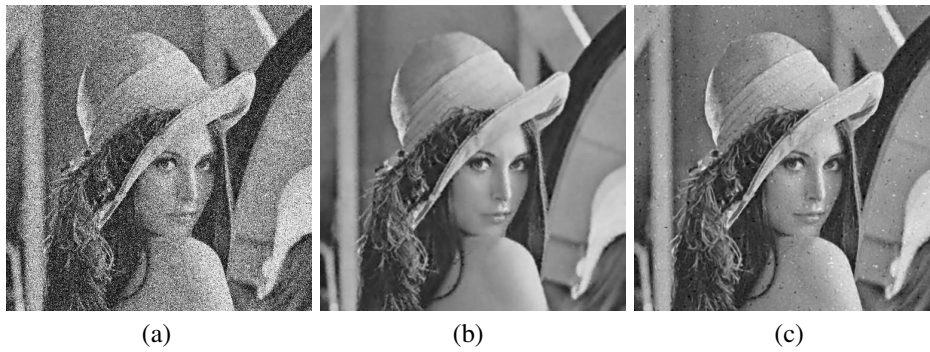
Fig. 7. (a) Lena corrupted by 50% of impulse noise of type II, (b) denoising using the kernel approach (PSNR=30.71 dB), (c) denoising with SKR - L_1 (PSNR=29.05 dB).
