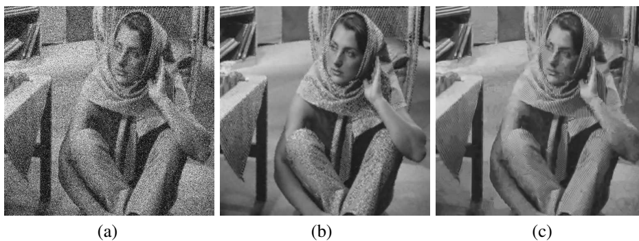
Fig. 8. (a) Barbara corrupted by 40% of impulse noise of type II, (b) denoising using the kernel approach (PSNR=24.81 dB), (c) denoising with BM3D (PSNR=27.05 dB).
