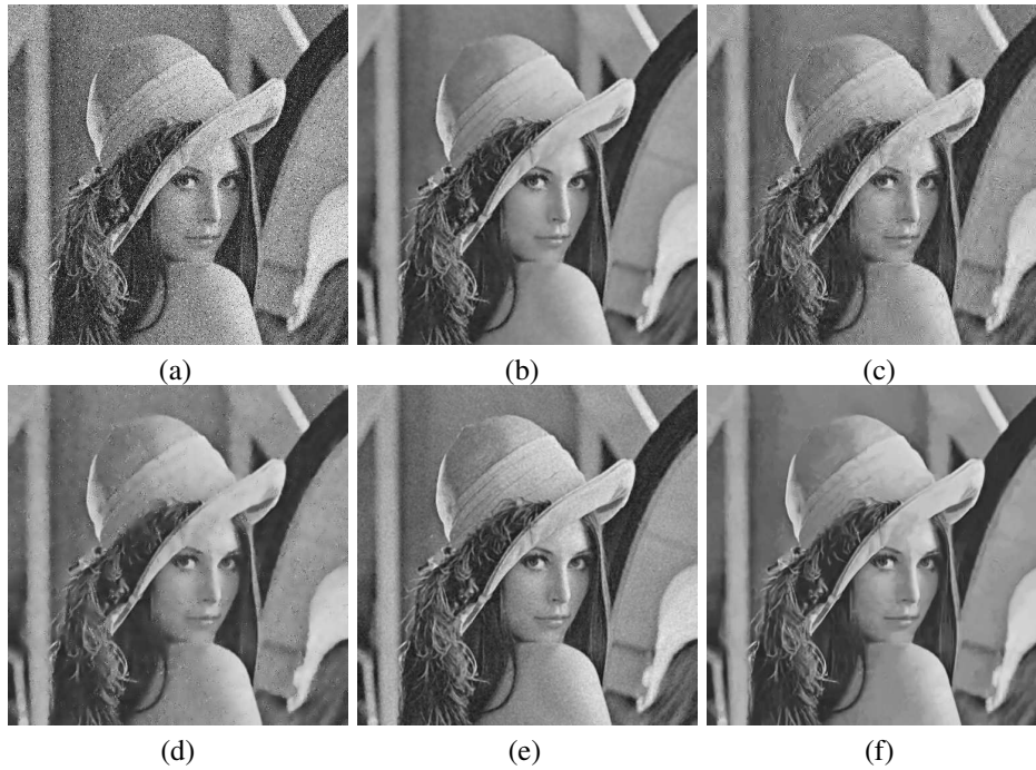
Fig. 12. (a) Lena corrupted by gaussian noise with s = 10 and 20% of impulse noise of type II ( a = 128 ), (b) denoising using the kernel approach (PSNR=32.27 dB), (c) denoising with BiShrink (PSNR=25.30 dB), (d) denoising with K-SVD (PSNR=27.51 dB), (e) denoising with SKR L_1 (PSNR=31.14 dB), (f) denoising with BM3D (PSNR=30.65 dB).
