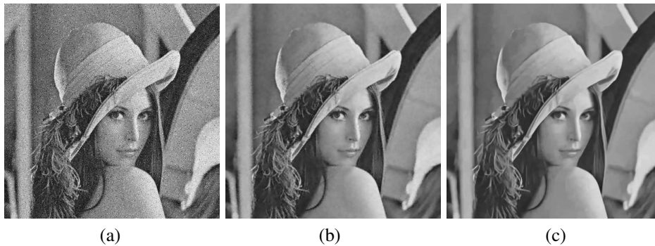
Fig. 14. (a) Lena corrupted by gaussian noise with s = 10 , uniform noise in the interval [-10, +10] and 10% of impulse noise of type II ( a = 128 ), (b) denoising using the kernel approach (PSNR=32.74 dB), (c) denoising with BM3D (PSNR=31.77 dB).
