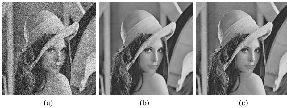
Fig. 6. (a) Lena corrupted by 40% of impulse noise of type II, (b) denoising using the kernel approach (PSNR=31.78 dB), (c) denoising with SKR - L_1 (PSNR=31.33 dB).
